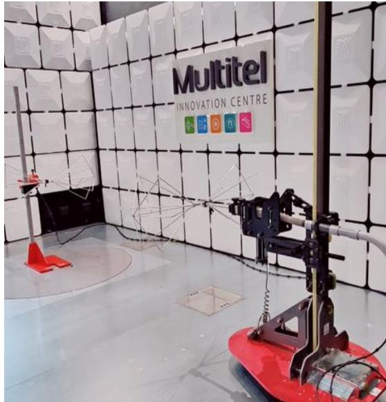
When in need of a new 3m EMC chamber, Multitel, a commercial EMC test lab, sought a solution partner to help develop their testing infrastructure. They desired a turnkey measurement system, including instrumentation, software, building preparation (concrete, HVAC, electrical), and long-term calibration support. The project was particularly challenging due to the limited space available in the parent building.
