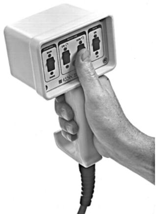
To connect the Hand Control Unit (HCU), remove the connector cap on the motor base. Plug the cable receptacle from the hand control unit into the electrical enclosure and screw connectors completely together. The HCU is now ready to operate. Be sure to coordinate use of the unit with the operator of the Model 2090 Positioning Controller.
