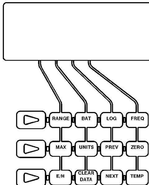
In some situations it may be helpful to fix the scale of the HI-3804. Press RANGE once to select the current scale setting. Each time you press RANGE the scale moves to the next least sensitive range. When the least sensitive scale is reached, it starts again at the most sensitive range.
